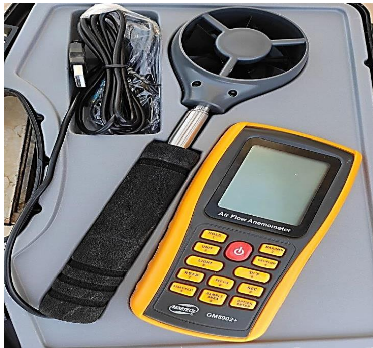
Fig.4.15. Air Flow Anemometer.
