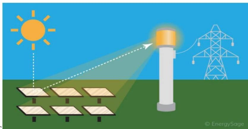
**Figure 1.1: Heliostat solar collector [1]**
