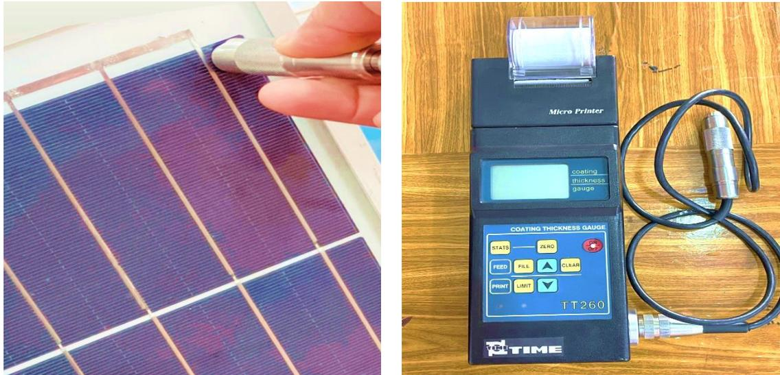
**Figure 3.8: Coating Thickness Gauge.**
