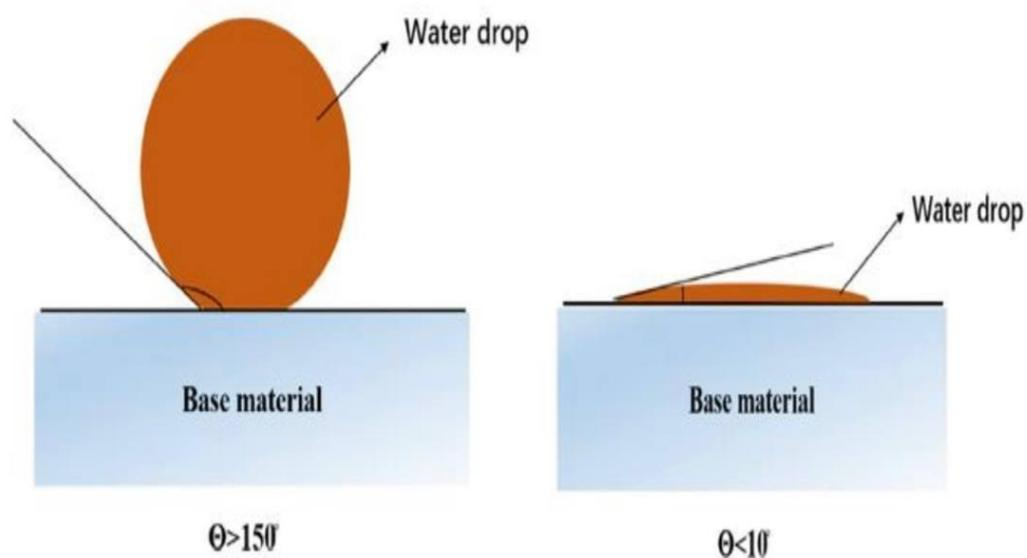
**Figure 2.1: Super-hydrophobic, Super- hydrophilic surfaces [25]**
