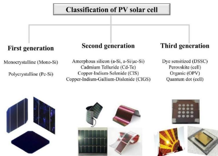
**Figure 1.4: Generational categorization of photovoltaic panels [5]**
