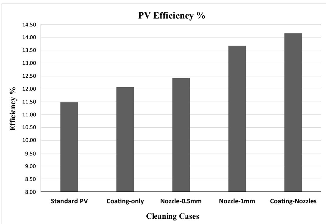
Figure 4.8: PV Efficiency for all cleaning cases-Day1
