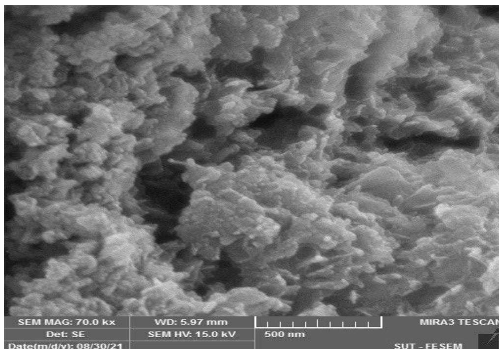
**Figure 4.2: FE-SEM for ZnO thin film at 220 mJ**
