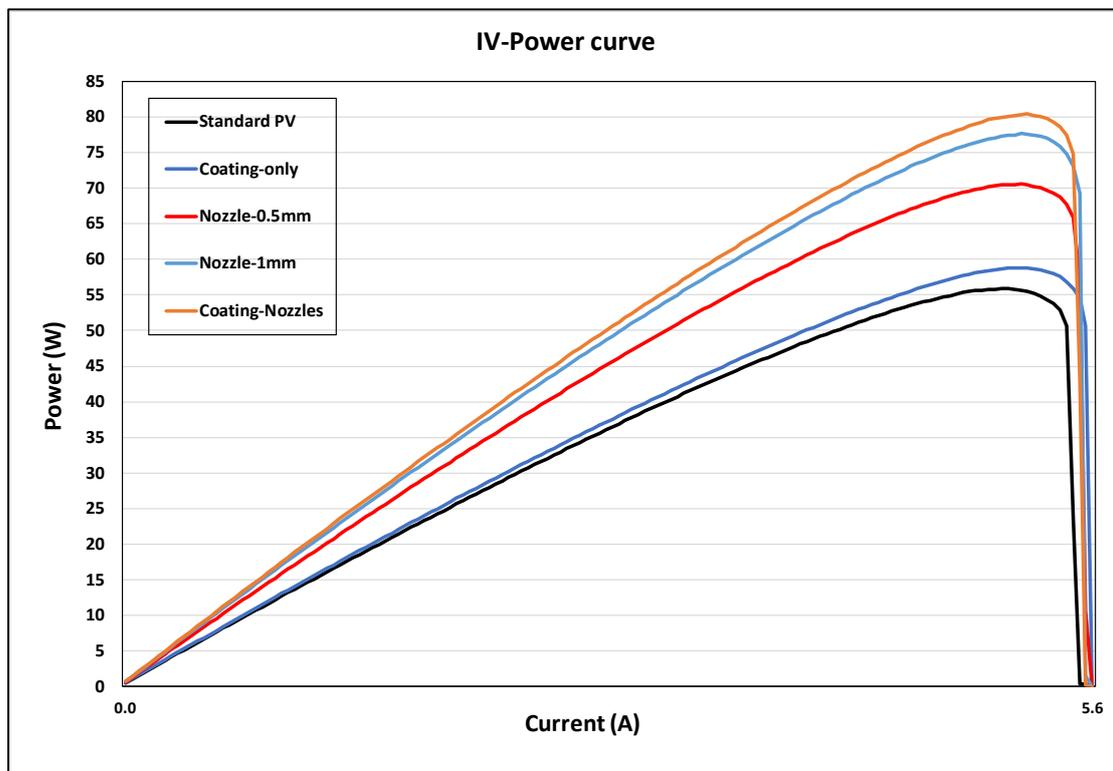
**Figure 4.16: PV output power for all cleaning cases-Day25**
