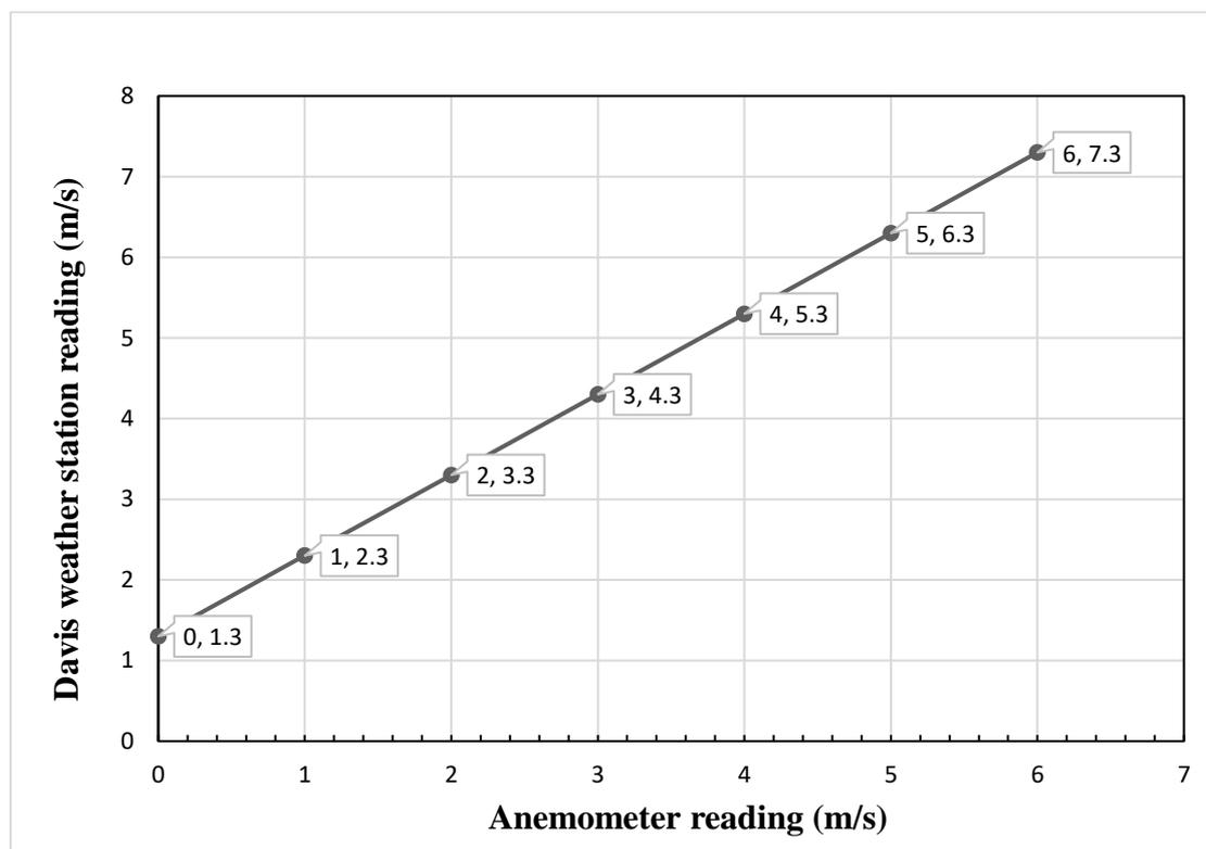
Figure B.2: Anemometer calibration with Davis weather station
