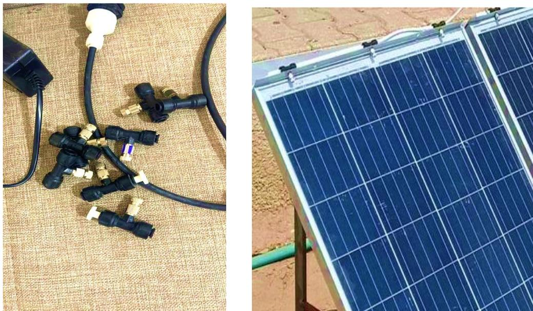
**Figure 3.3: Water nozzles used to spray water on the PV.**
