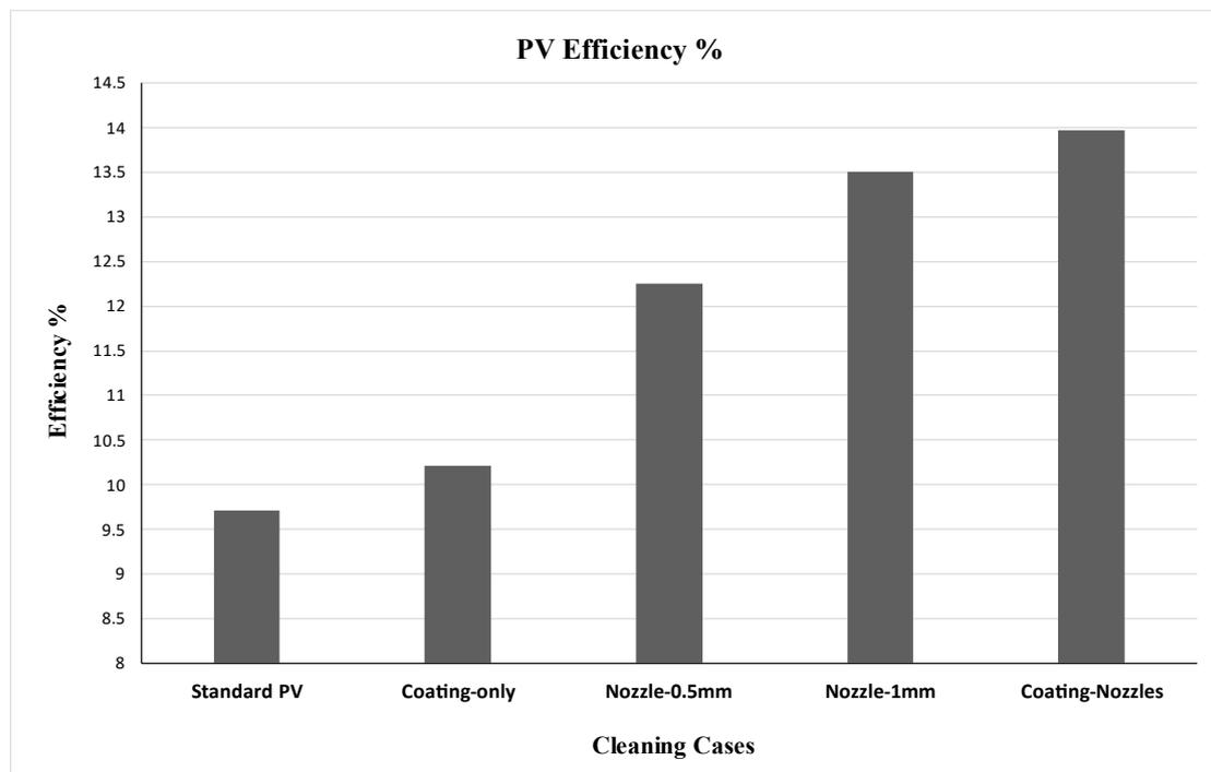
Figure 4.18: PV Efficiency for all cleaning cases-Day25
