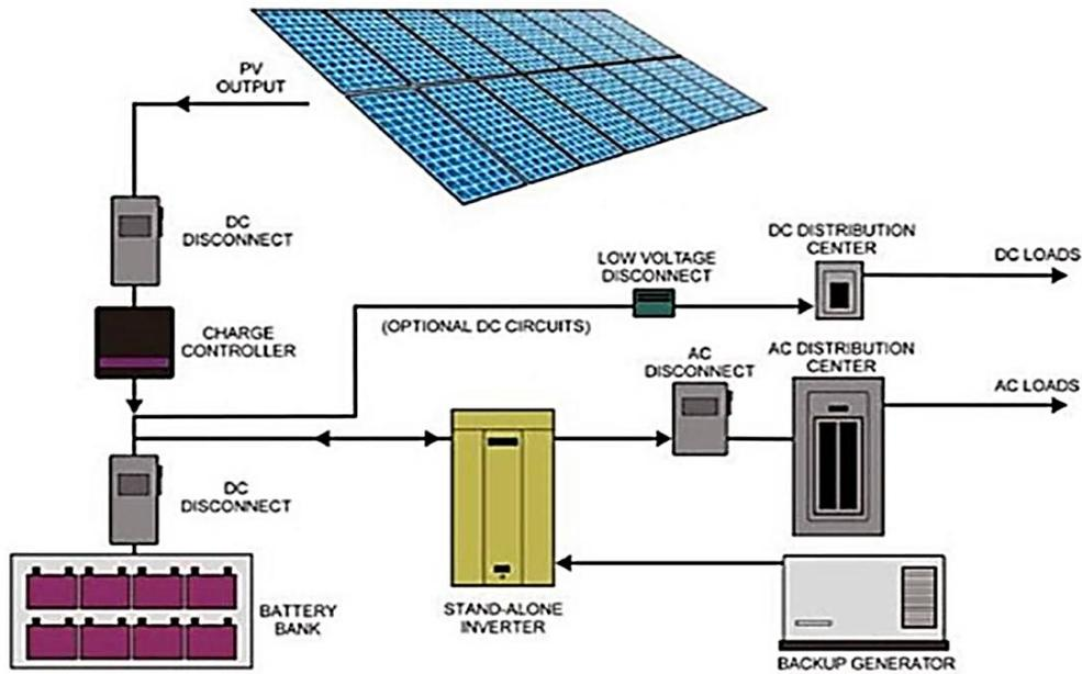
**Figure 1.3: photovoltaic panel installation [3]**
