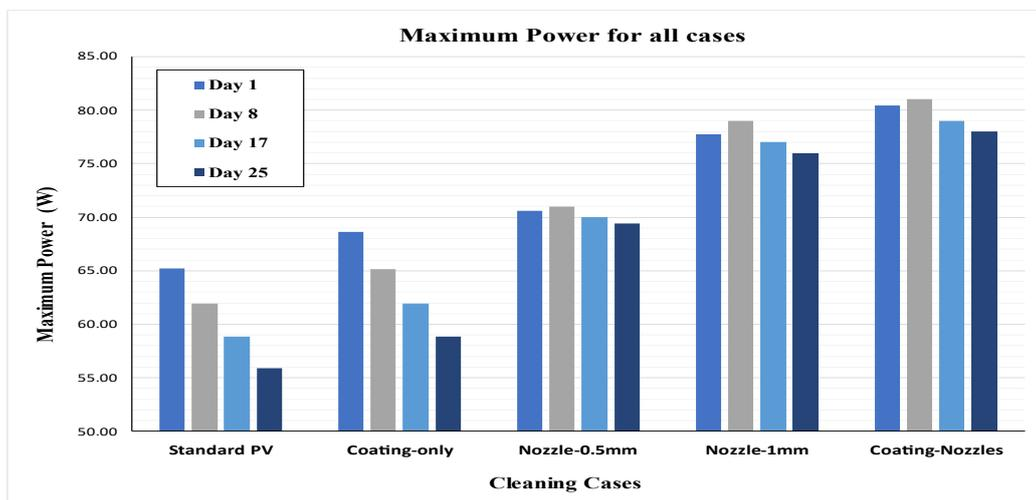
Figure 4.21: PV power output for all days and cleaning cases
