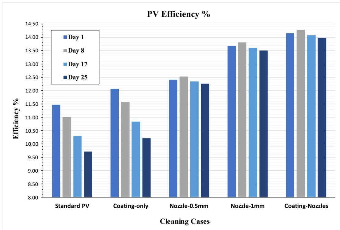
Figure 4.20: PV Efficiency for all days and cleaning cases
