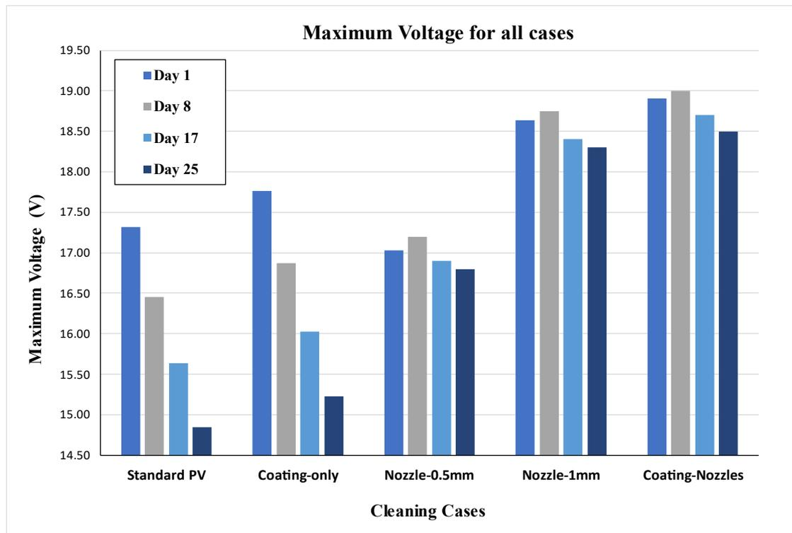
**Figure 4.22: PV voltage for all days and cleaning cases**
