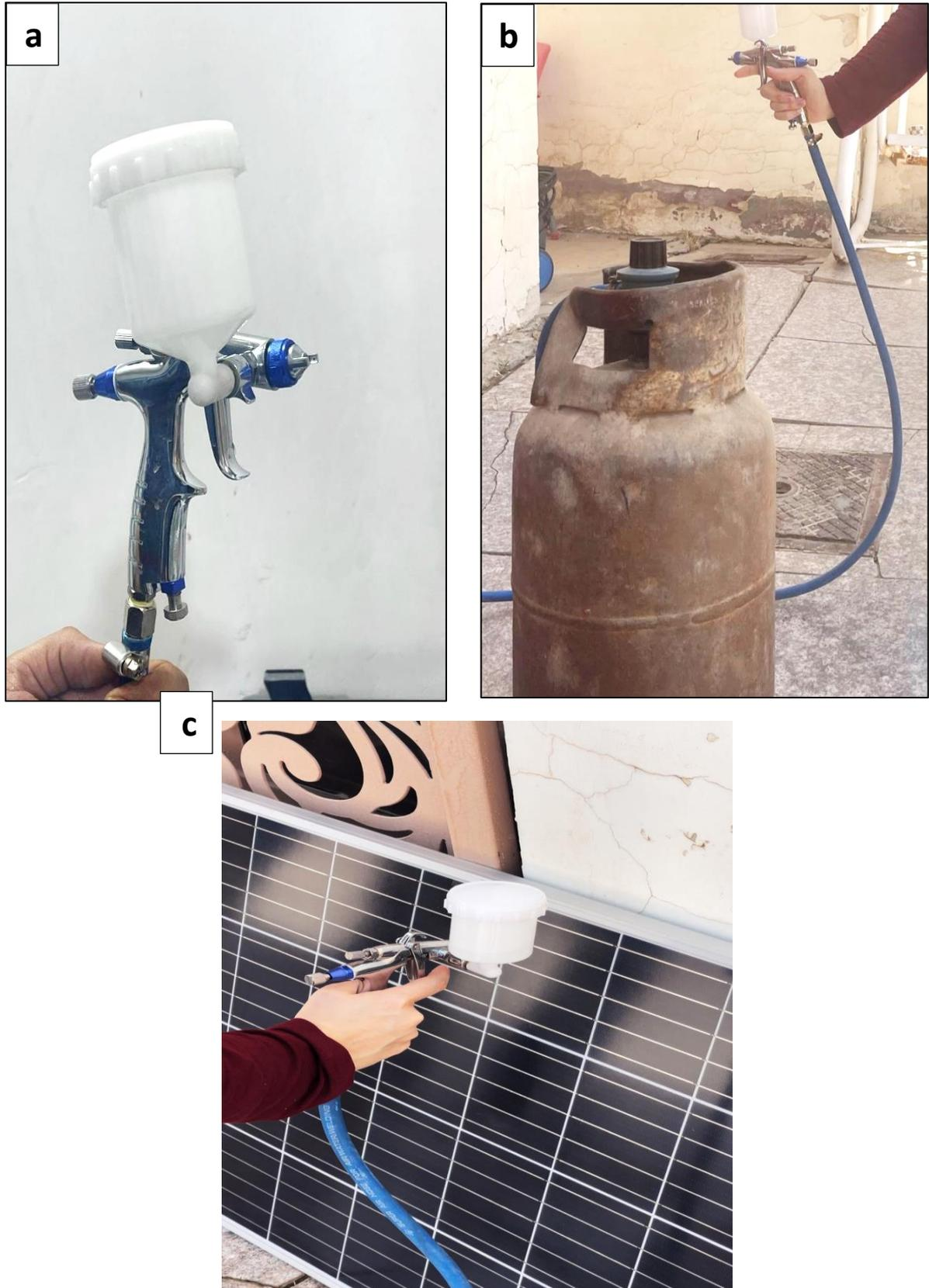
Figure 3.6: (a, b, and c) Illustration of coating process
