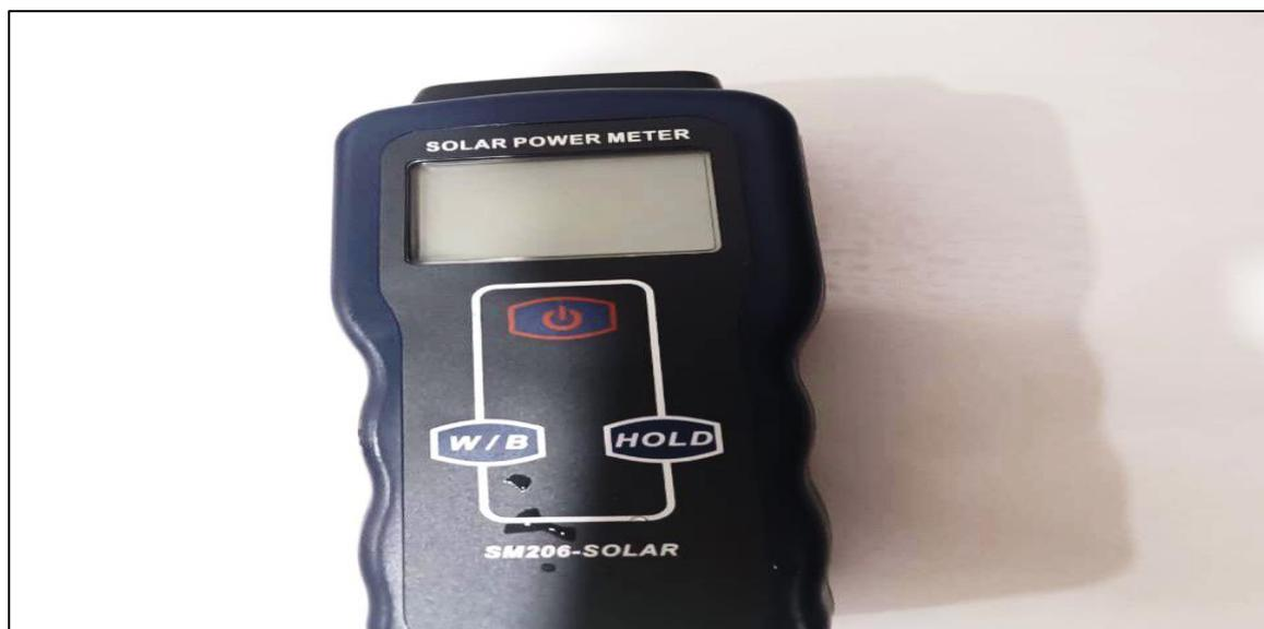
**Figure 3.9: Solar Power Meter.**
