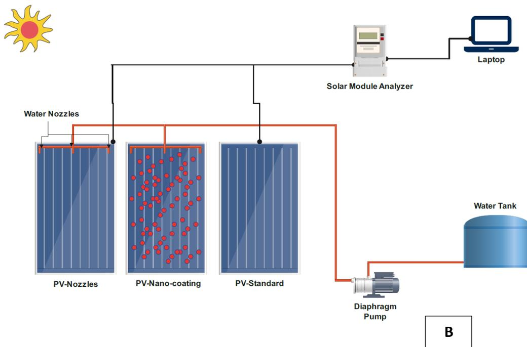
**Figure 3.12: A: Experiment setup, B: Blueprint diagram**
