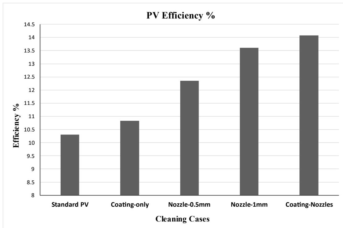
Figure 4.14: PV Efficiency for all cleaning cases-Day17
