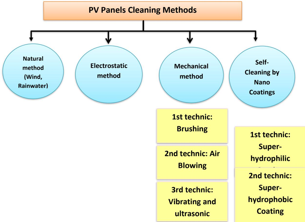
**Figure 1.9: PV Panels Cleaning Methods**
