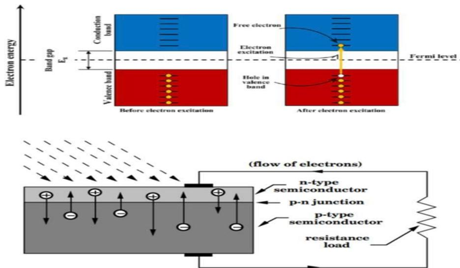
**Figure 1.5: Solar cell operation [10]**
