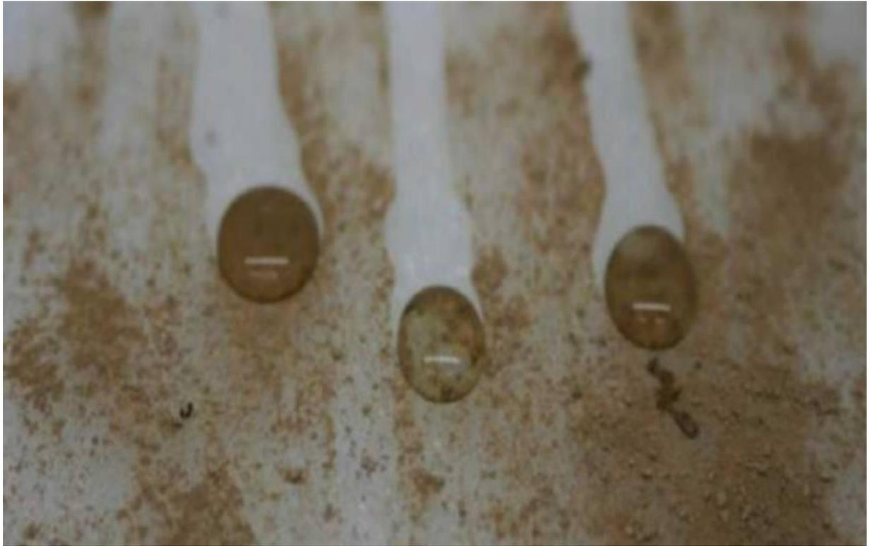
**Figure 2.2: Water droplets flowing down the superhydrophobic surface carrying dust particles [26].**
