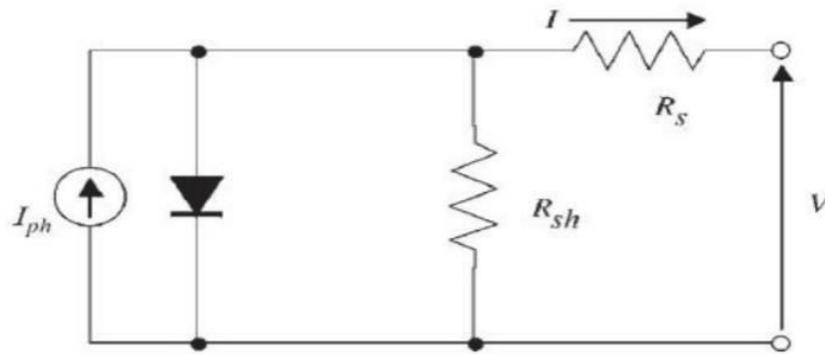
Figure 1.6: Photovoltaic cell electrical diagram[11]
