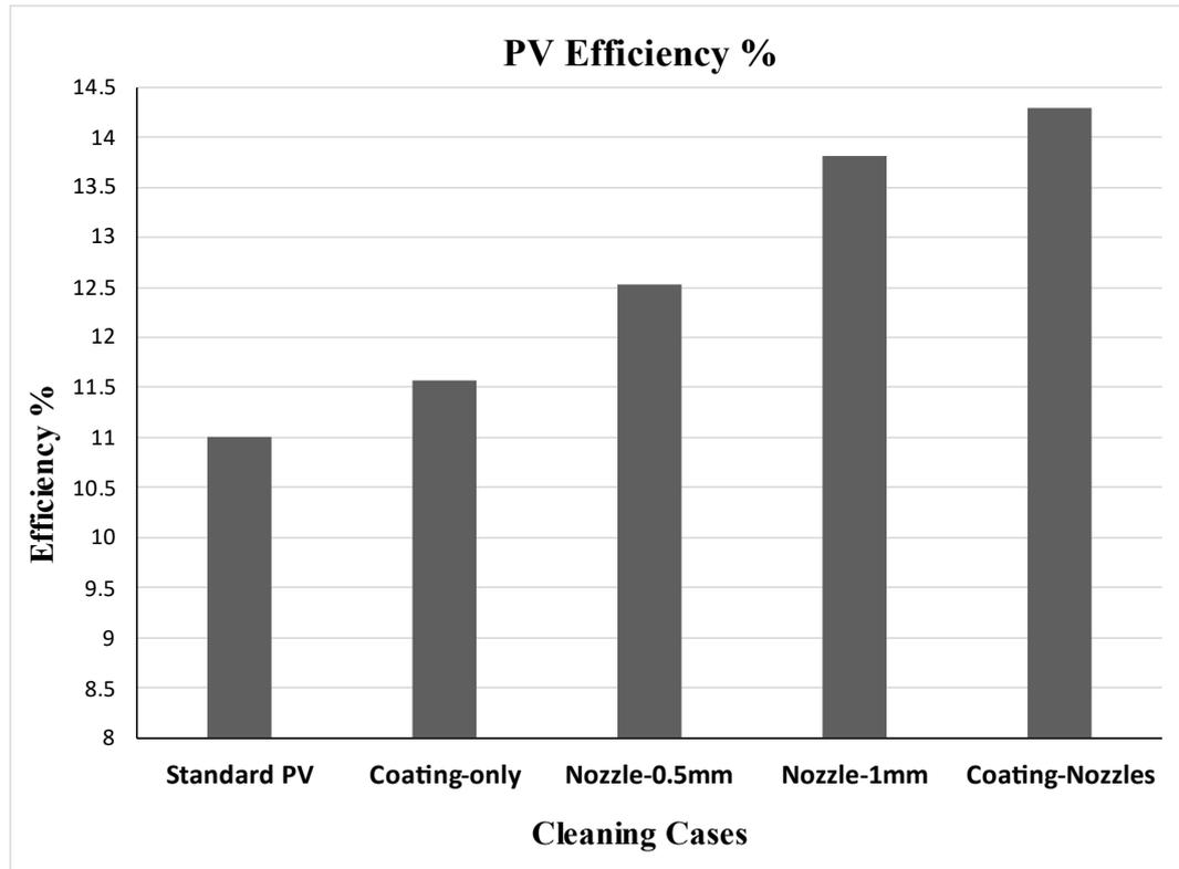
Figure 4.11: PV Efficiency for all cleaning cases-Day8
