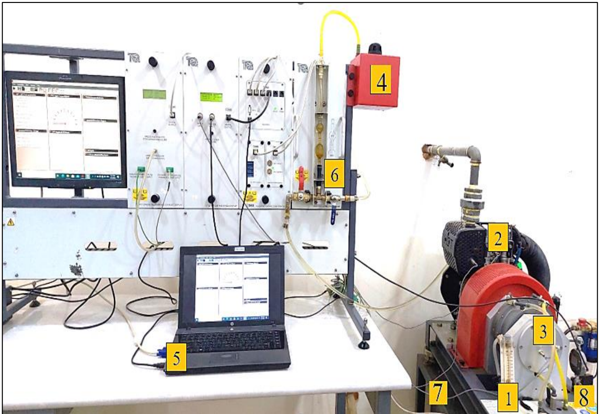
1-Flowmeter 2-CI Engine 3- Dynamometer 4- Fuel tank 5- computer 6- Volumetric fuel gauge 7- Air box 8- Torque sensor (load cell)
