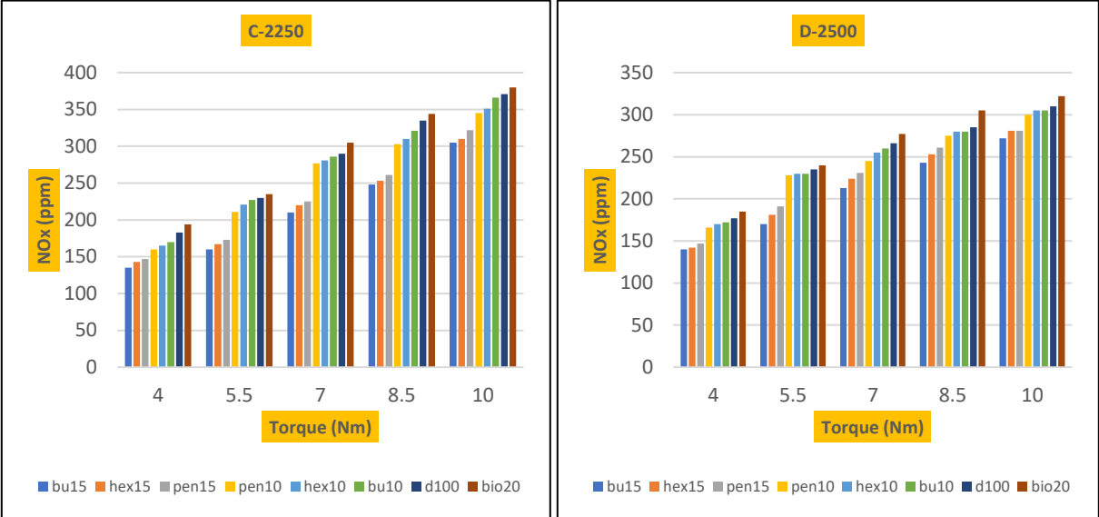
Figure (4-10): Variation of Nitrogen of Oxides (NOx) depending on engine loads.
