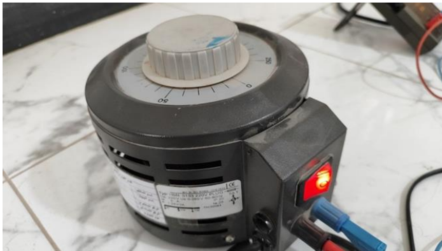
Figure ( 4-4 ) The Variable Transformer
