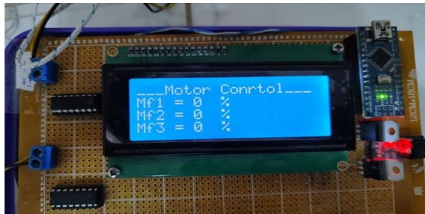
Figure ( 4-7 ) Fan speed regulator
