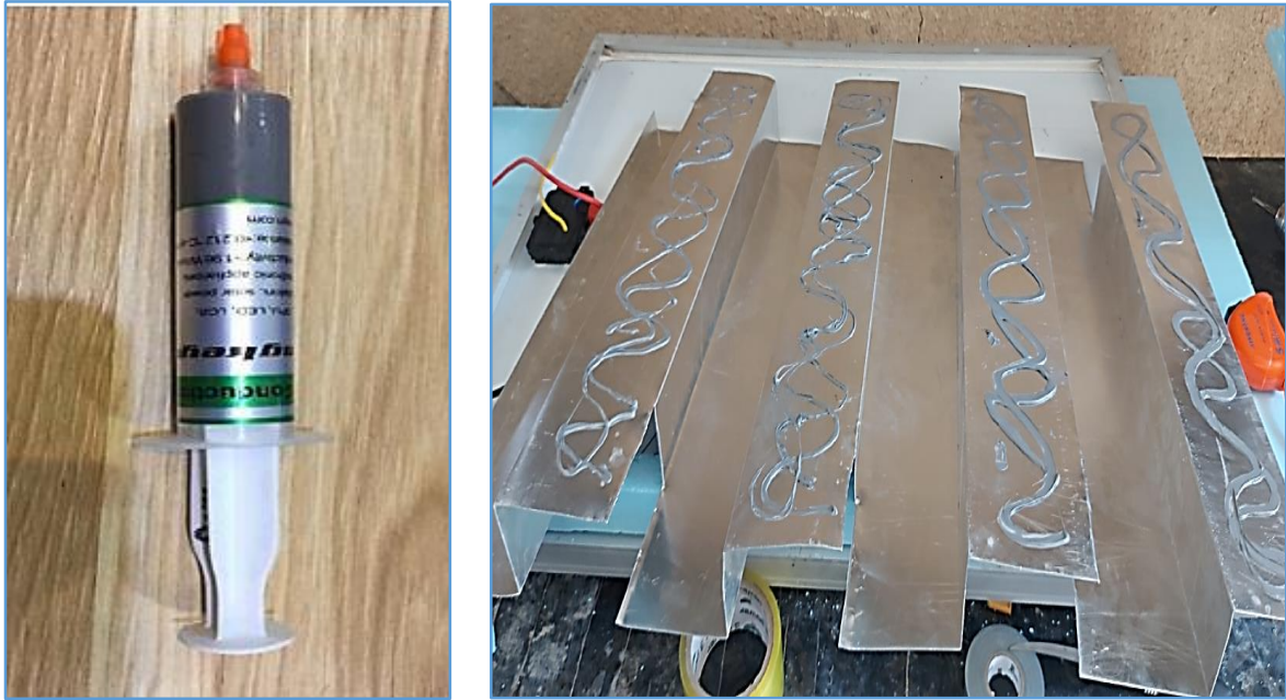
(a) (b) Figure (4.5). (a) Thermal paste. (b) Multi-flow channel.
