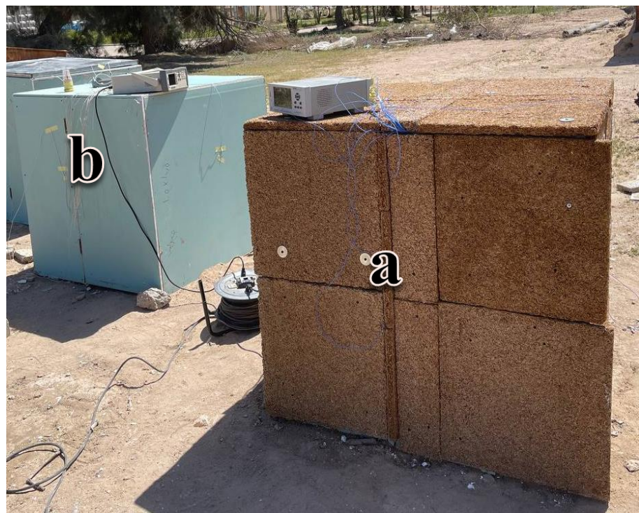
Figure 3-10 (a) Test room that is covered with insulating materials (b) Test room without insulation
