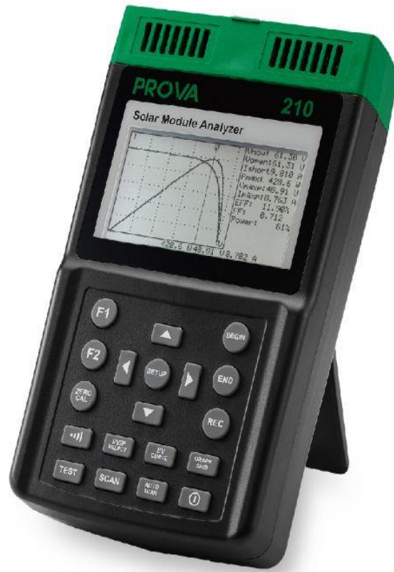
Figure 4.20. PV Analyzer device.
