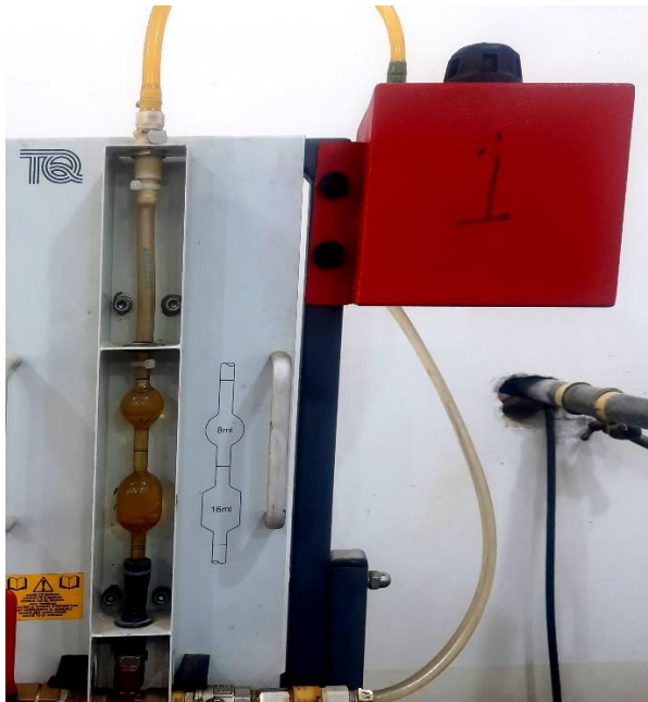
Figure 3.12 Volumetric fuel meter.
