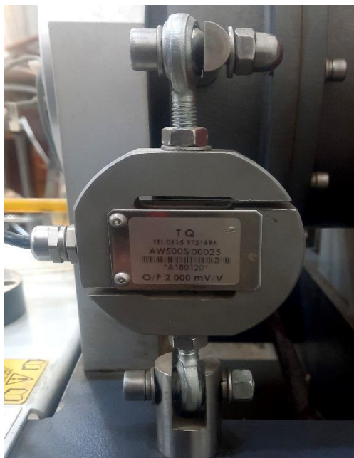
Figure 3.9 torque sensor (load cells).
