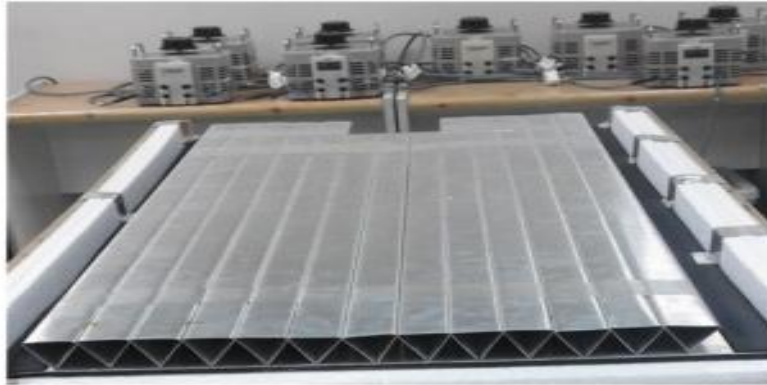
Figure 2-4 V-corrugated absorber plate air system [18].
