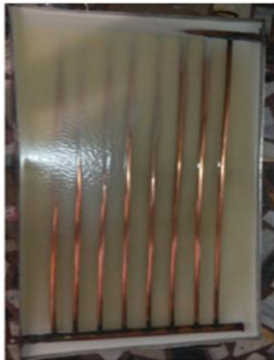
Figure2- 14 PV/T with PCM and copper pipes [30].
