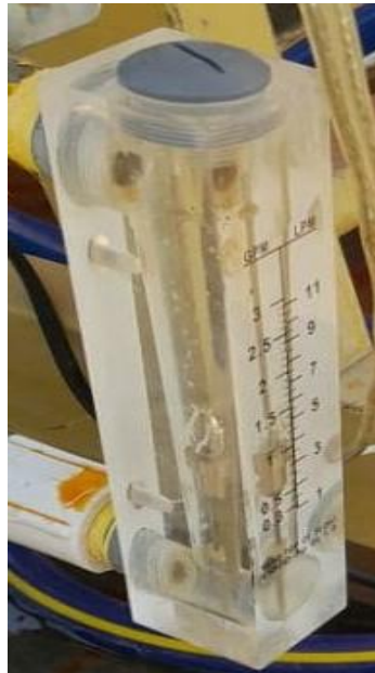
Figure 4-13AM-4206M Flow meter device
