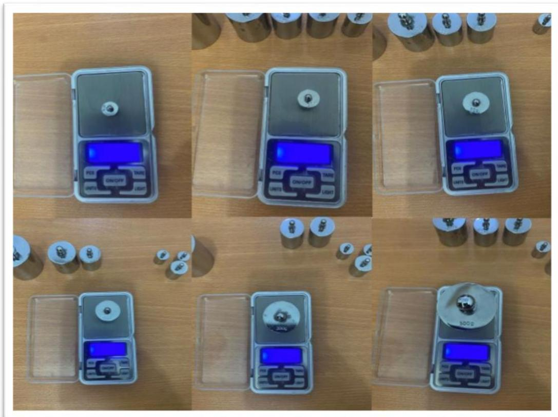
Figure D-2: Photograph for the calibration of a device
