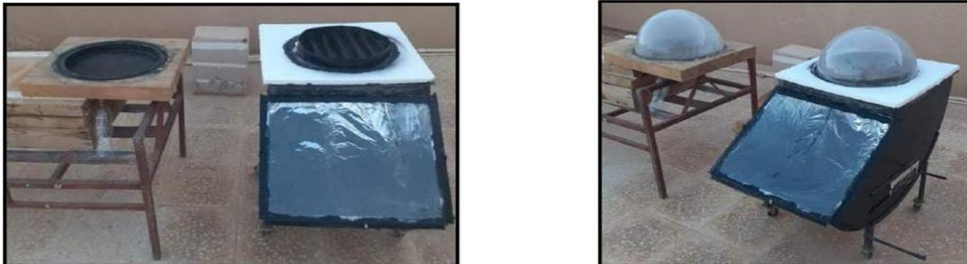
a) Traditional hemispherical solar still (THSS) and hemispherical solar still with a sinusoidal liner incorporated with an inverted solar collector (SHSS-ISC)
