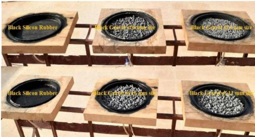
**Figure (2.3):** View of the basin of hemispherical distillers with black gravels [13].
