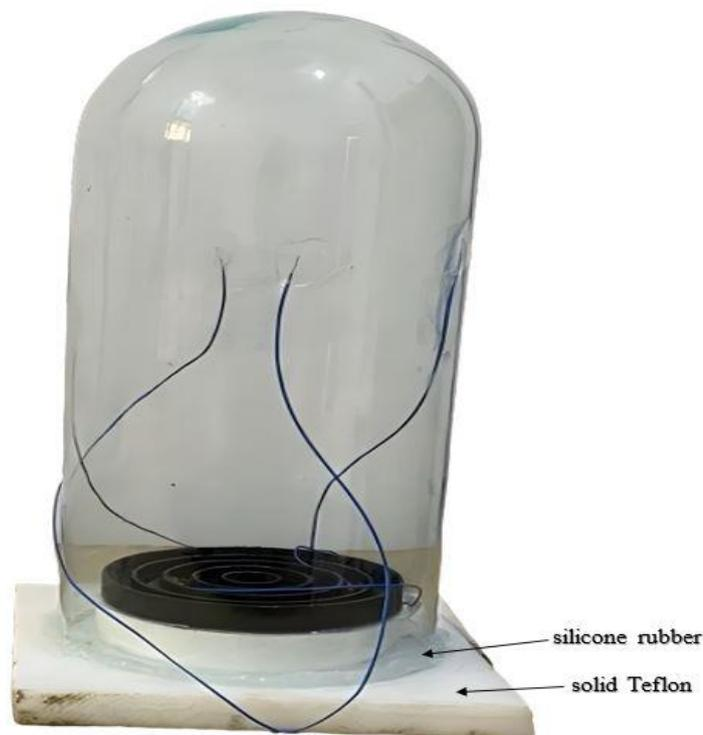
**Figure (4.5):** Photograph displaying the sealant used in a solar still.
