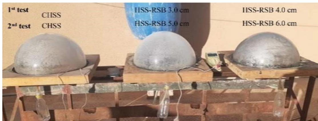
**Figure (2.10): (b)** Photograph depicting a basin with rock salt balls arranged at varying intervals of 3.0, 4.0, 5.0, and 6.0 cm [23].
