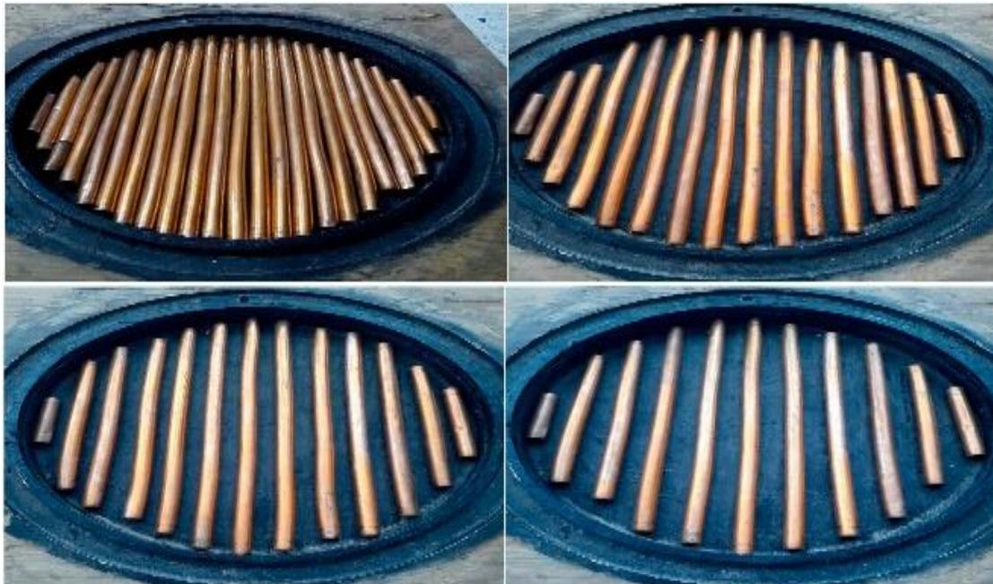
**Figure (2.12):** Photo of EHCF position inside distilled basin with the change of the distance between them (0, 2, 3, and 4 cm) in order [26].
