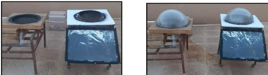
b) Traditional hemispherical solar still (THSS) and hemispherical solar still with a half-circle liner incorporated with an inverted solar collector (HCHSS-ISC)
