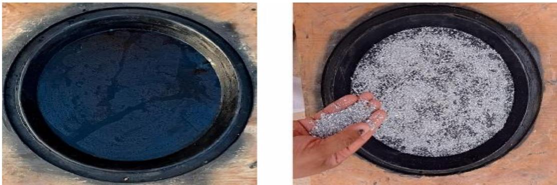
Figure (2.22): (a) A photograph of the hemispherical solar still basin without and with aluminum waste [36].
