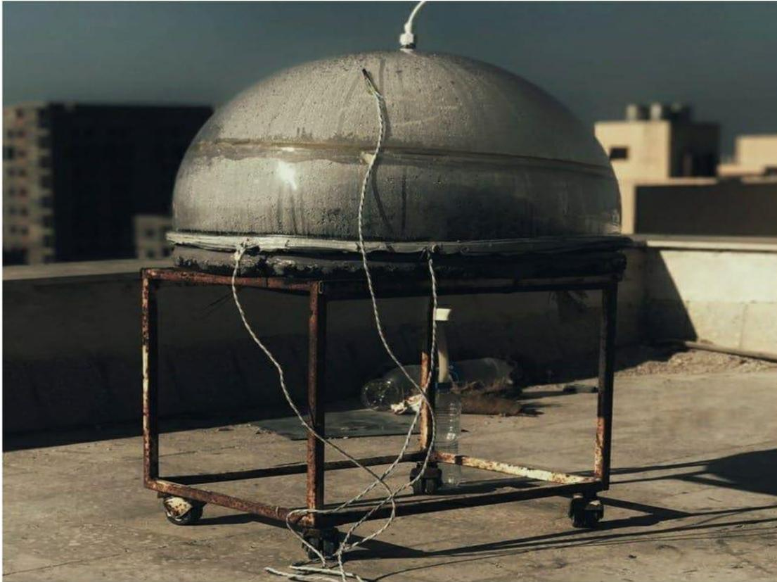
**Figure (2.17):** Photo of tested dish solar still (DSD) [31].
