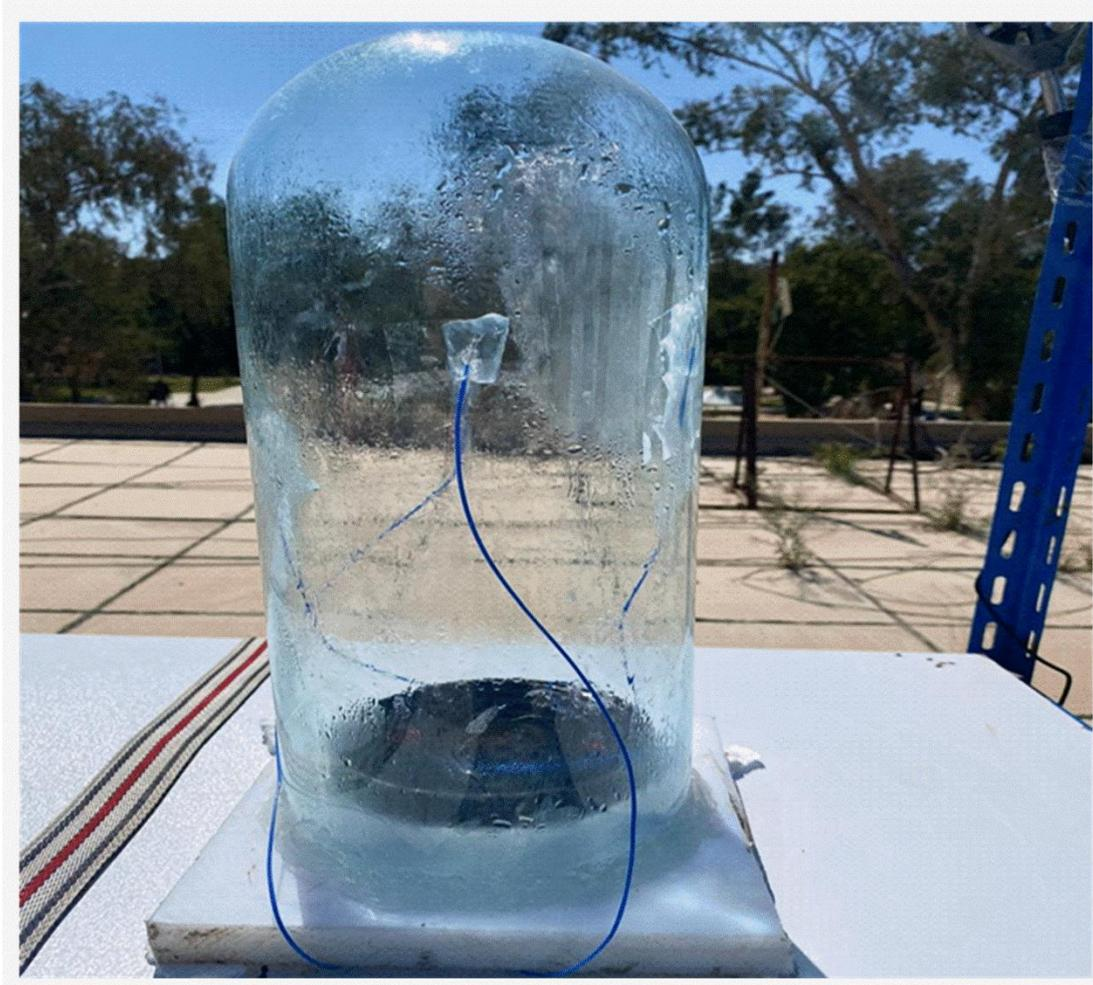
**Figure (4.4):** Photographic view of solar still glass cover
