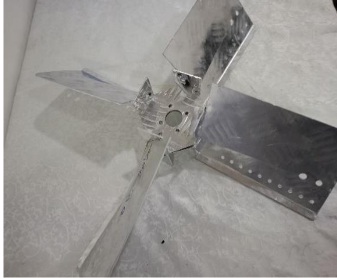
Figure 3.9 fan M7clockwise fan made of aluminum
