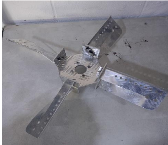
Figure 3.7 M5 clockwise fan made of aluminum
