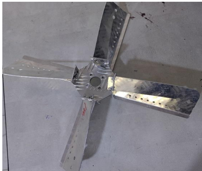
Figure 3.8 fan M6 clockwise fan made of aluminum
