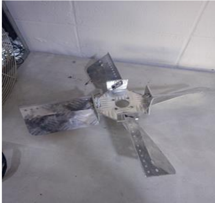
Figure 3.4 Fan M2 counterclockwise made of Aluminum
