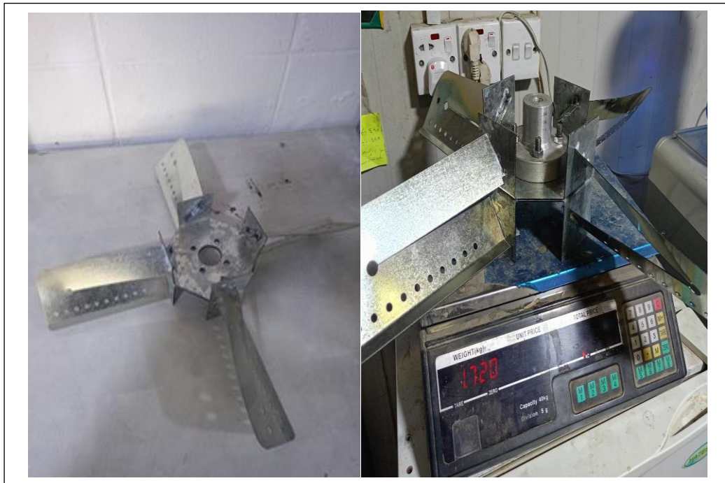
Figure 3.3 fan M1 counterclockwise made of galvanized iron
