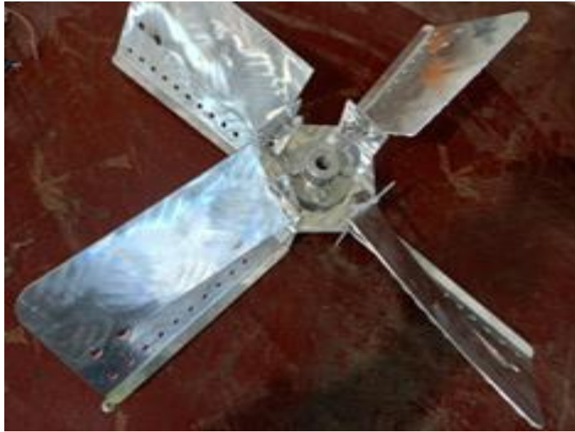
Figure 3.6 Fan M4counterclockwise made of aluminum
