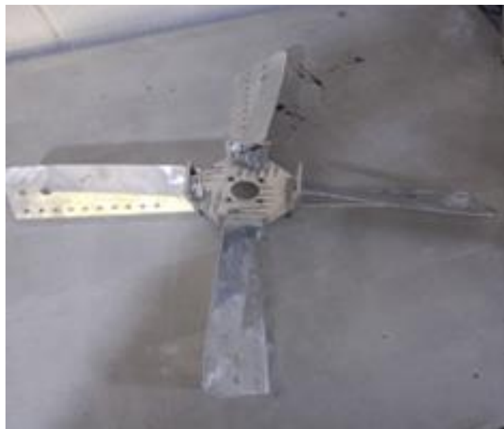
Figure 3.5 Fan M3 counterclockwise made of Aluminum
